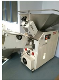
BA02 Pietroberto Omega 3 volumetric divider Capacity: 250kg Pieces weights: 100g-1600g Output: 1200-2400 pieces/hr
