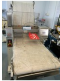
BA05 Pietroberto semi-auto dough Sheeter Belt width: 600mm Belt length: 2300mm
