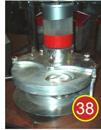
38 Semi-automatic hamburger press. 1300 pieces per hour
