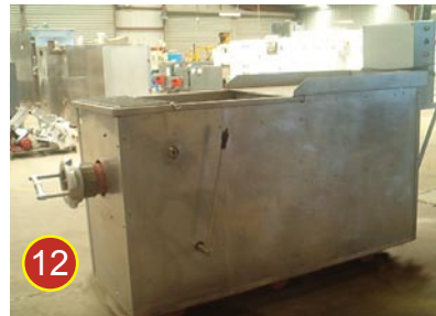
12 VVS mincer mod.180. Output: 4000kg/hr approx. Suitable for frozen products & mortadella.
