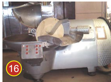
16 Kramer-Grebe bowl cutter. Capacity: 380L approx. Very good condition. Output: 6000-7000kg/hour.
