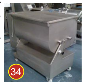
34 Meat mixer with double paddle NEW! Capacity 180kg.
