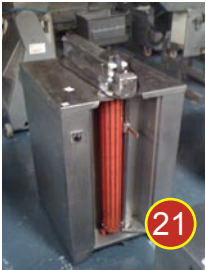
21 Lead machine for smallgoods. Puts metal label on salami, prosciutto etc.
