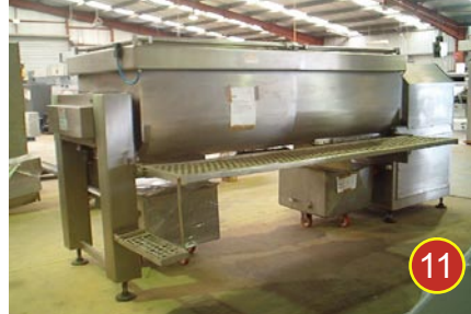
11 Velati mixer 2500L approx NEW! With discharge under tank. Stainless steel construction. Vacuum optional.
