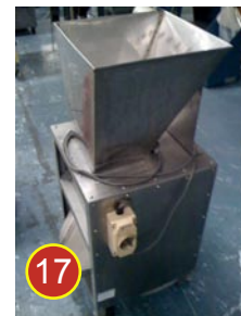
17 Small strips cutter for steaks, cabbage etc.. For strips of 30mm up to 120mm. Approx 1000-1500kg/hr.
