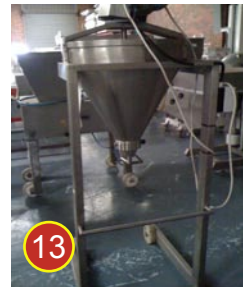
13 Velati salt-spreader. Works as part of an automatic line.
