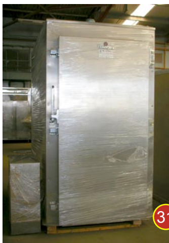
31 Travaglini TZ oven with separate smoke generator. Capacity: 2 trolleys, 1000kg product approx. Trolley dimensions: 2.0m (h) x 1.0m x 1.0m. With computer control. The best system for steam cooking meat, fish, chicken etc.
