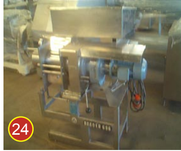
24 Baader 696 meat separator for poultry.
