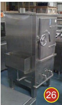
26 J.Curtin steam autoclave. Stainless steel. Gas model. Capacity: 50kg approx.
