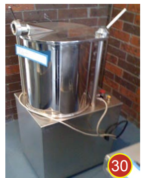
30 Vertical hydraulic sausage filler (NEW) . 50L capacity.
