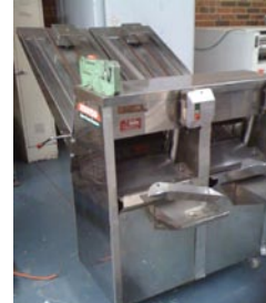
#51 Mono twin bread slicer. 300mm + 300mm. One side slices 9mm, one side slices 13mm.
