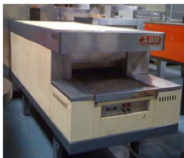
#41 Rinaldi SuperABO tunnel oven for pita bread, Arabic bread, and other middle-eastern products. Max temperature 600 degrees C.
