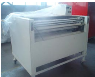
#38 Bertrand resting machine. With felt pockets for 32 portions 50g to 1200g.
