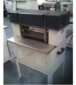
#47 Gasparin slicer 400mm. Thin only (9mm).
