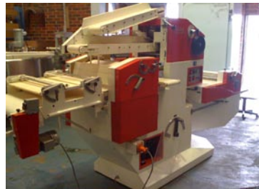
#35 Sottoriva automatic group complete with rounder. Pieces from 35g-920g approx.
