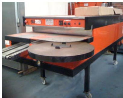
#42 Rinaldi "Superpizza" electric tunnel oven. Loading & unloading from front.
