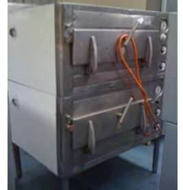
#5 Sterlec electrical oven. 2 decks. With brick base in cooking chamber.
