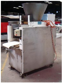
#29 Winkler volumetric divider. Pieces from 30g to 1200g. Hopper capacity: 60kg.
