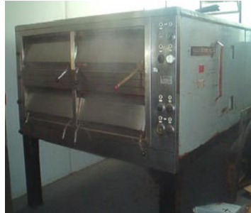
#8 Les Wilson electrical oven. 2 decks, Baking area: 8.26m 2 . With brick base in cooking chamber.
