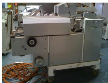
#56 APV slicer 300mm. Slices 11mm only.
