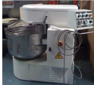
#61 Tecnopast spiral mixer. 80kg finished dough approx.
