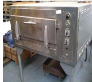
#4 Sterlec electrical oven. Baking chamber dimensions: 90 x 160cm. With brick base in cooking chamber.
