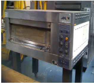
#2 Sveba-Dahlen electrical oven. 1 deck.
