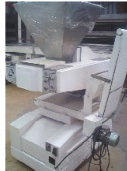
#36 Bertuetti volumetric divider. Pieces from 80g to 1600g.
