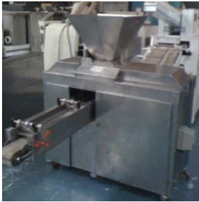
#30 Mono volumetric divider. Pieces from 50g to 1500g. Hopper capacity 80kg.
