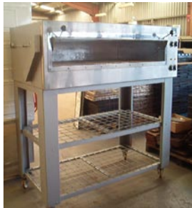
#7 Electra-Bake electrical oven. 1 deck. Brick base.
