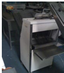
#53 MEC slicer 400mm. Slices 16mm/10mm.
