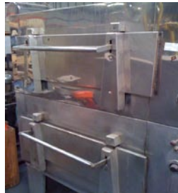
#3 Pyroseal electrical oven. 2 decks, 6 trays (45 x 75cm). With brick base in cooking chamber.
