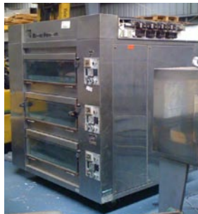
#13 Baker-Perkins "Rotel" rotary oven. Suitable for 12 trays.
