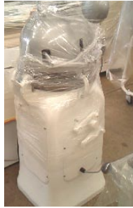
#31 Eberhardt rounder/divider. Pieces from 30g to 140g. Max dough: 3600g
