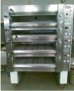
#1 Electro-Dahlen electrical oven. 4 decks, 8 trays (45 x 75cm).
