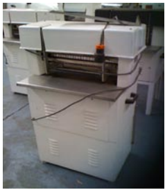
#48 Gasparin slicer 500mm. Thick & thin (10mm/12mm)
