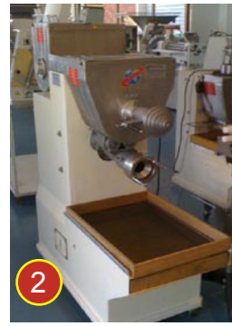
2 La Parmigiana D55DV double hopper extruder (USED). 35kg/hr approx.
