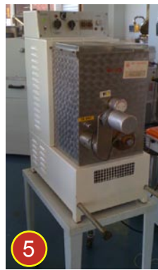
5 Eidelweiss extruder (USED). 25kg/hr approx.
