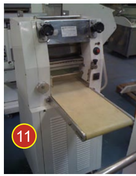
11 Dominioni long pasta cutter. Sheet width: 250mm. With interchangeable dies.
