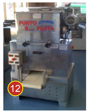
12 Dominioni double bowl cylinder/sheeter. Sheet width: 250mm approx. Output: 180kg/hr approx. USED but in very good condition.
