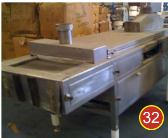
Cozzi steam pasteuriser. 4m long approx. Belt width: 470mm. (AS NEW)
