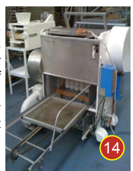
12 Dominioni double bowl cylinder/sheeter. Sheet width: 250mm approx. Output: 180kg/hr approx. USED but in very good condition.
