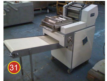
Toresani horizontal pasta cutter (AS NEW). With 3 cuts: lasagne, fettuccine 7, linguine. Sheet width: 300mm approx.
