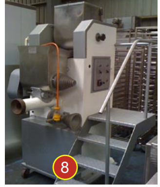
8 La Parmigiana D80N double bowl extruder (USED). Output: 60-70kg/hr approx. With fan to pre-dry pasta.
