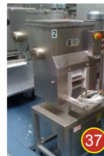
LB double bowl cylinder/sheeter (AS NEW). Sheet width: 160mm approx.
