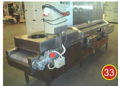
Horizontal pasta cutter (USED). With 4 cuts: lasagne, fettuccine 7, linguine, spaghetti. Sheet width: 400mm approx.
