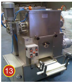
13 Dominioni double bowl cylinder/sheeter. Sheet width: 280mm approx. Output: 200kg/hr approx. AS NEW!
