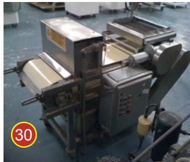
Horizontal pasta cutter (USED). With 4 cuts: lasagne, fettuccine 7, linguine, spaghetti. Sheet width: 400mm approx.
