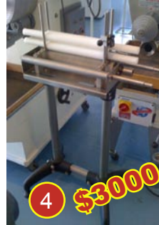
4 La Parmigiana sheet winder (NEW). Rolls up sheet from extruder ready for use in other machines. $3000
