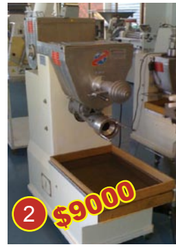
2 La Parmigiana D55DV double hopper extruder (USED). 35kg/hr approx. $9000
