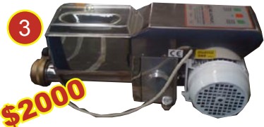
3 Bottene extruder (NEW). Output: 5-6kg/hr approx. Ideal for small restaurants and cafes. Stainless steel. $2000
