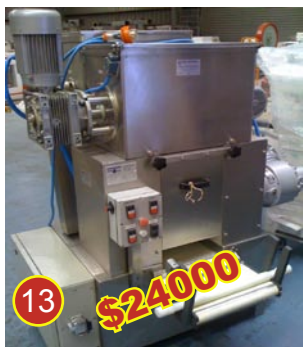
13 Dominioni double bowl cylinder/sheeter. Sheet width: 280mm approx. Output: 200kg/hr approx. AS NEW! $24000
